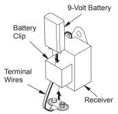
Figure 16 - Installing Battery in Receiver
